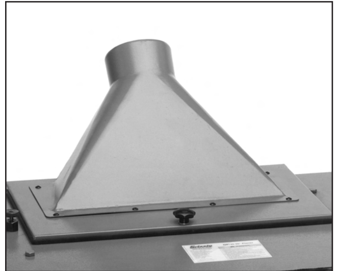
Figure 4. Dust hood installed.
